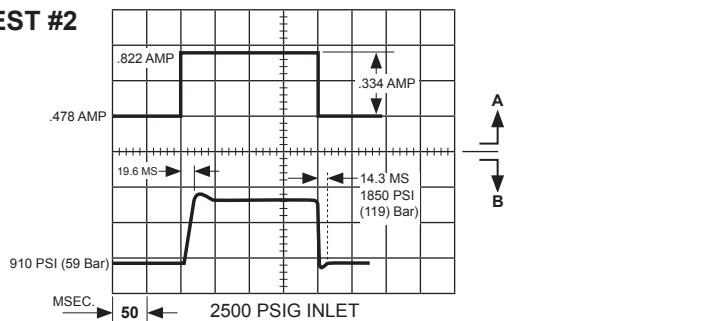
**Note:** Test data shown is with a "C" size reducer at 2500 PSI.
